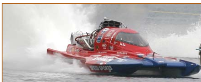
Lou Osmond's Speed Sports Top Fuel Drag Hydroplane. -2007 World Champion. World Record Holder -4.7ET at 255.6MPH, uses Ferrea Super Alloy Exhaust and Ferrea Titanium intake valves.
